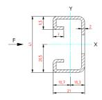
Maximum deflection / force calculated based on max. allowed bending stress
