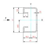
Maximum deflection / force calculated based on max. allowed bending stress
